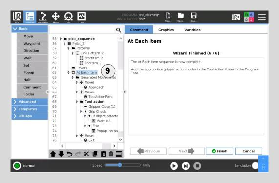
9 Once the tool action is complete, the next move is an exit point.
