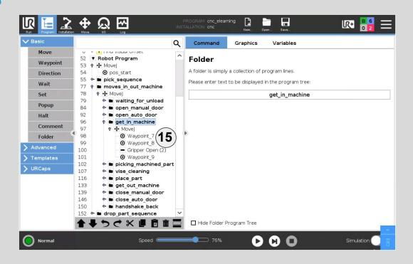
The next **folder** is used to get the robot in position for picking the completed part. The first two points are used to get over the part with the second gripper.
