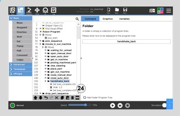
When everything is done, the robot sends the signal to the machine to start it's machining process.
