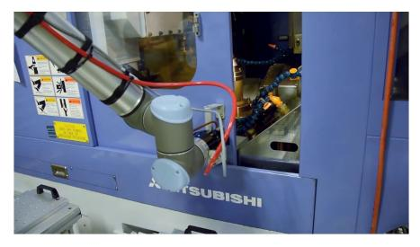
The major advantages of this solution are simplicity and cost effectiveness. In fact, if you own a robot you also own a CNC machine door opener. There is no need for a robot/machine handshake and you can be up and running in no time.
