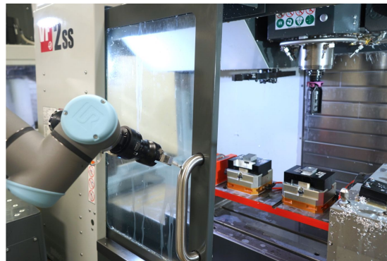
Fig 1.1 Cobot Opening a CNC Machine Door
